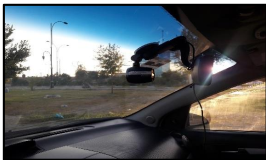
Fig. 2: Dash Camera Mounted in Windshield of Test Car
